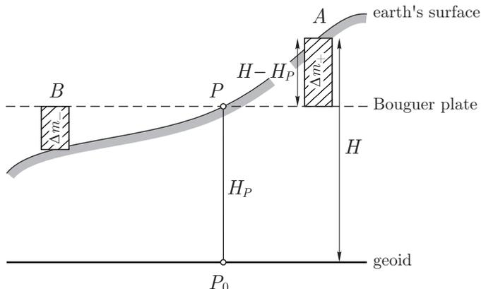
Fig. 3.6. Terrain correction
