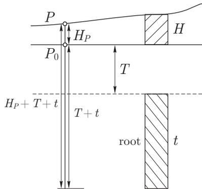
Fig. 3.12. Topography and compensation – Airy–Heiskanen model
