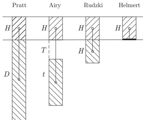
Fig. 3.16. Topography and compensation for different gravity reductions
