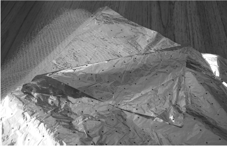
Figure 9.17: A section of multilayered insulation, with one layer folded back to reveal the nylon bridal veil spacer. Each layer is perforated with small holes, spaced at approximately 1-cm intervals, to allow trapped air to escape from the layers.
