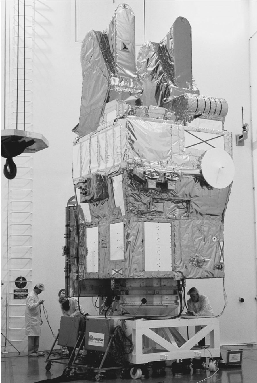
Figure 9.15: The SPOT 5 Earth-observation satellite. The thermal control subsystem design governs the way the spacecraft looks. (Image copyright © CNES/Patrick Dumas.)
