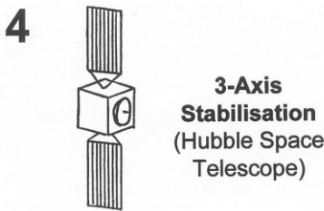
Figure 8.3: The four general types of spacecraft attitude stabilization. All spacecraft fall into one of these categories, some examples of which are illustrated. (Image credits: Meteosat SG image, copyright © ESA; Intelsat 6 image, copyright © Boeing; GPS Navstar 2R image, copyright © Lockheed Martin; Hubble Space Telescope image, copyright © NASA.)
