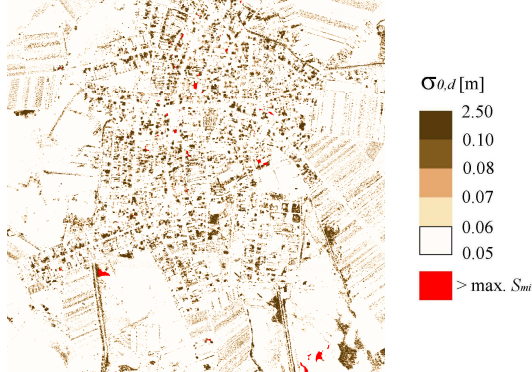
Figure 5) has an a-priori defined lower limit, which in this case is 5cm. It is determined regarding to post-processing steps, which include quality checks and fine georeferencing of ALS strips. The best accuracy is reached where the terrain is flat and without vegetation or big buildings (area with fields).
