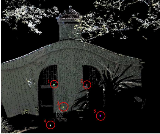
Figure 2. Control Points seen in the point cloud from the first scan point.
