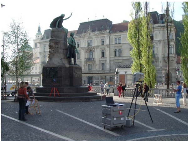
Figure 6. Terrestrial laser scanning of the Prešeren's Monument, the monument to the greatest Slovenian Poet France Prešeren, The Prešernov square, Ljubljana.
