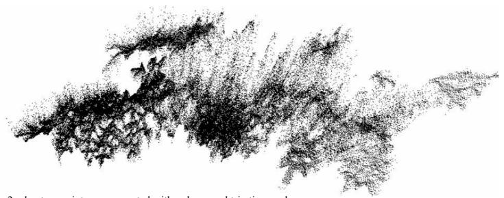
2: phantom points are generated with pulse round trip time and phased based distance measurement scanners.
