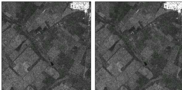
ENVISAT ASAR AP (HH polarization) multi-looked unfiltered (left) and Gamma-Gamma MAP filtered image (right). Note the speckle reduction while preserving the structural features of the Gamma-Gamma MAP one.
