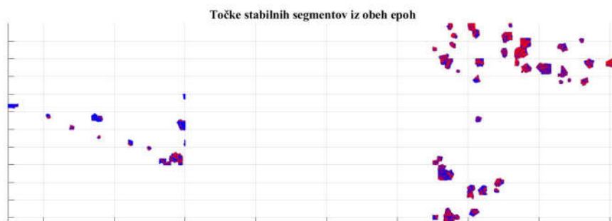
Figure 7: Points that lie within the most stable segments: first epoch in blue and second epoch in red
