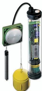
Float-operated Thalimedes shaft encoder Ott
