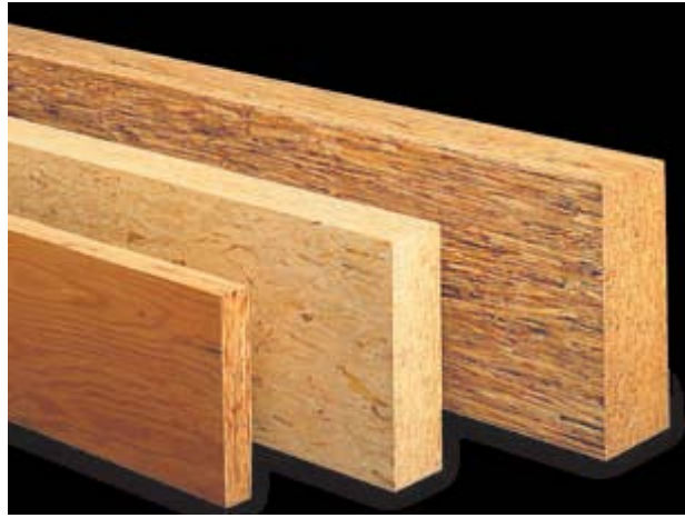
Konstruktivski kompozitni les (Z leve proti desni: Laminated Veneer Lumber – LVL, Laminated Strand Lumber – LSL, Parallel Strand Lumber – PSL)
